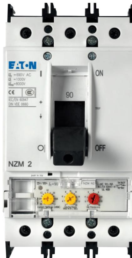
**Figure 3: The motor protective circuit breaker NZM2-ME-NA, listed per UL 489 and certified per CSA-C22.2 No. 5-09, has additionally been evaluated per the motor overload calibration requirements of UL 508 and CSA-C22.2 No. 14. In addition to the adjustable overload and instantaneous short circuit trip adjustments, the device has a motor inrush trip class selection feature similar to the ones available in premium design overload relays.**
