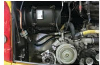
The FC800 EverCool refrigeration hose offers the necessary flexibility to allow for the relative movement between the compressor and hoses when the engine starts and allows for installation in space restrictive applications, due to its excellent bend radius.
